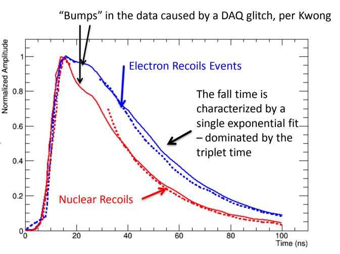
Solid Lines – 78 keV recoils in xenon with 60 V/cm from Kwong et al  $2009_3$ Dotted lines – NEST simulation with same physical parameters
